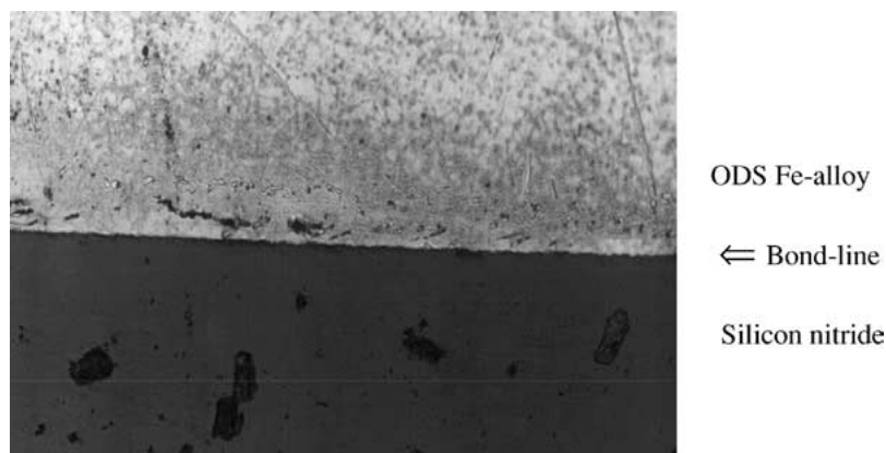
Figure 1 Light micrograph showing a transverse section through the TLP bonded ceramic-metal joint.
